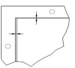
**6.** Seal the space between the frame and the wall with a silicone sealant.
