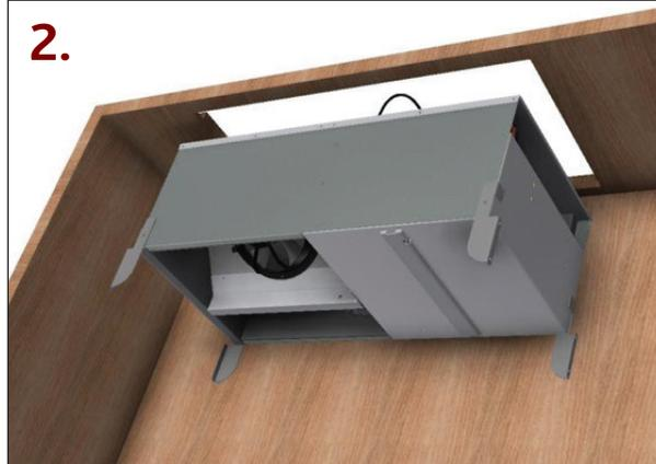
*Engage the conditioning unit in the cut-out space*
