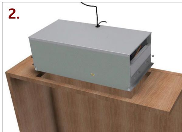
*Insert the unit into the cut-out space from above*
