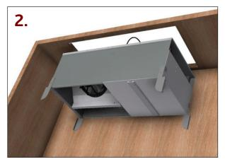
Engage the conditioning unit in the cut-out space
