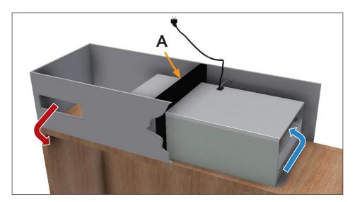
Separate the air flows. The free passage area of each grille is 200 cm<sup>2</sup>. Separation A is not supplied. Ensure the separation is adequately sealed.
