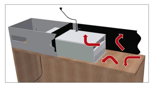
Additional sound insulation can be installed. This is particularly useful for the suction on all walls.
