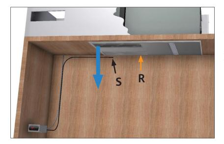
The thermostat can be installed in the cabinet, on the side of the cabinet or outside the cabinet. Its sensor (S) should be positioned towards the return air zone (R). We recommend that the end of the sensor does not touch the partition and is situated in the air flow.
