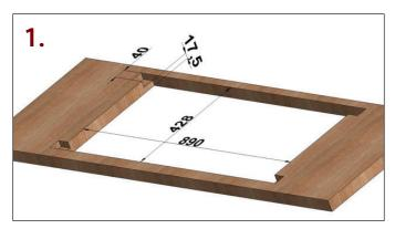
Cut the ceiling and adjust the slots for the legs if these are used
