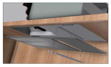
The hood is inserted on the left at the point of the slots and then screwed in. The cover is magnetic.
