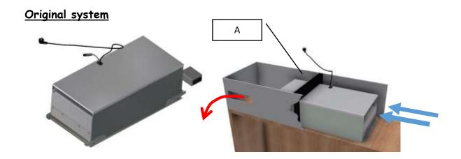
The free cross-section of each grid is  $200 \text{ cm}^2$ . Separation "A" is not provided. **Be sure to seal this separation.**
